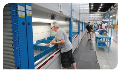
The PPG client handling module keeps each customer's inventory separate in the system, but not *physically* separate – providing the benefits of greater storage density and batch picking for faster order fulfillment.
